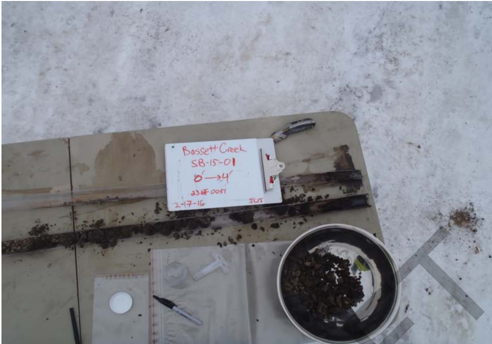
Photo 2: Geoprobe Core at SB-15-01
