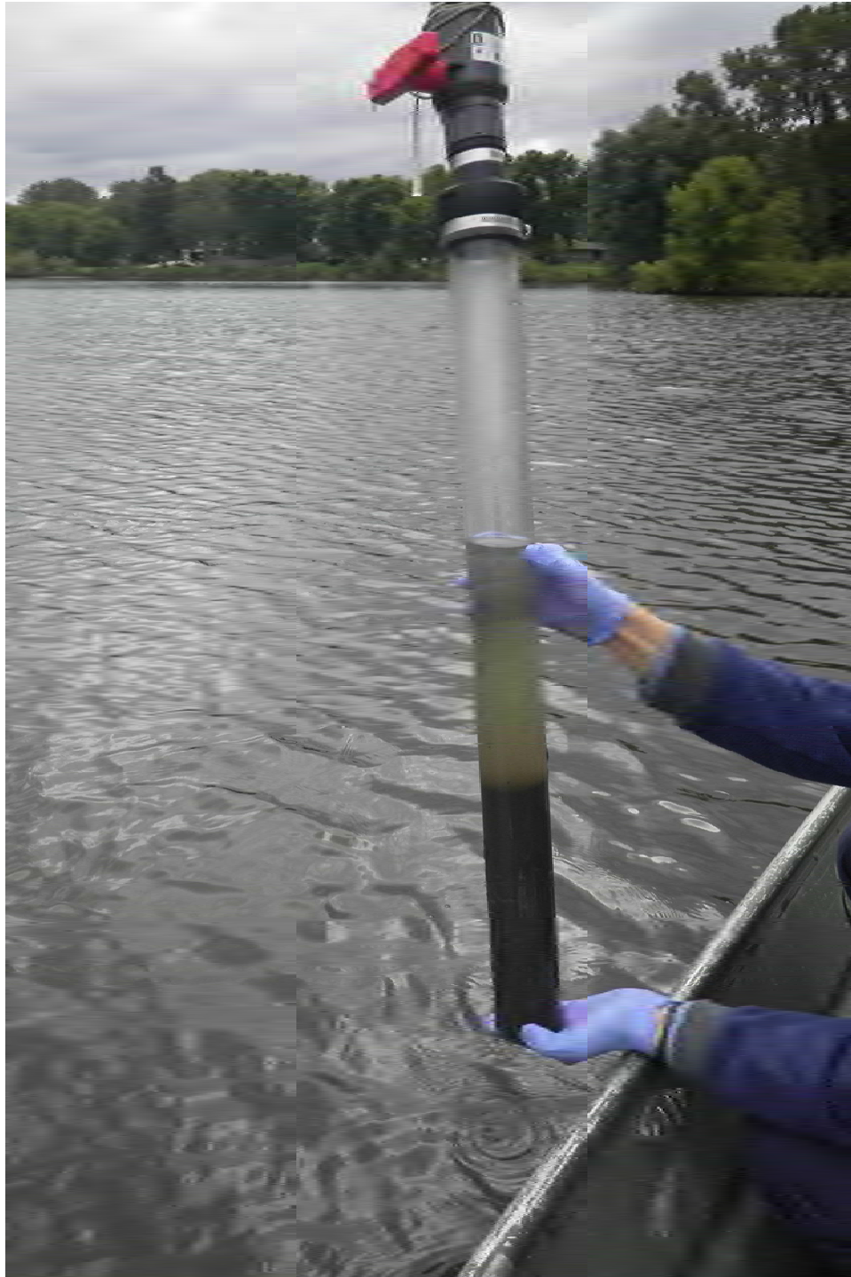
Photograph #1: Sediment core collected with push core sampling device.
