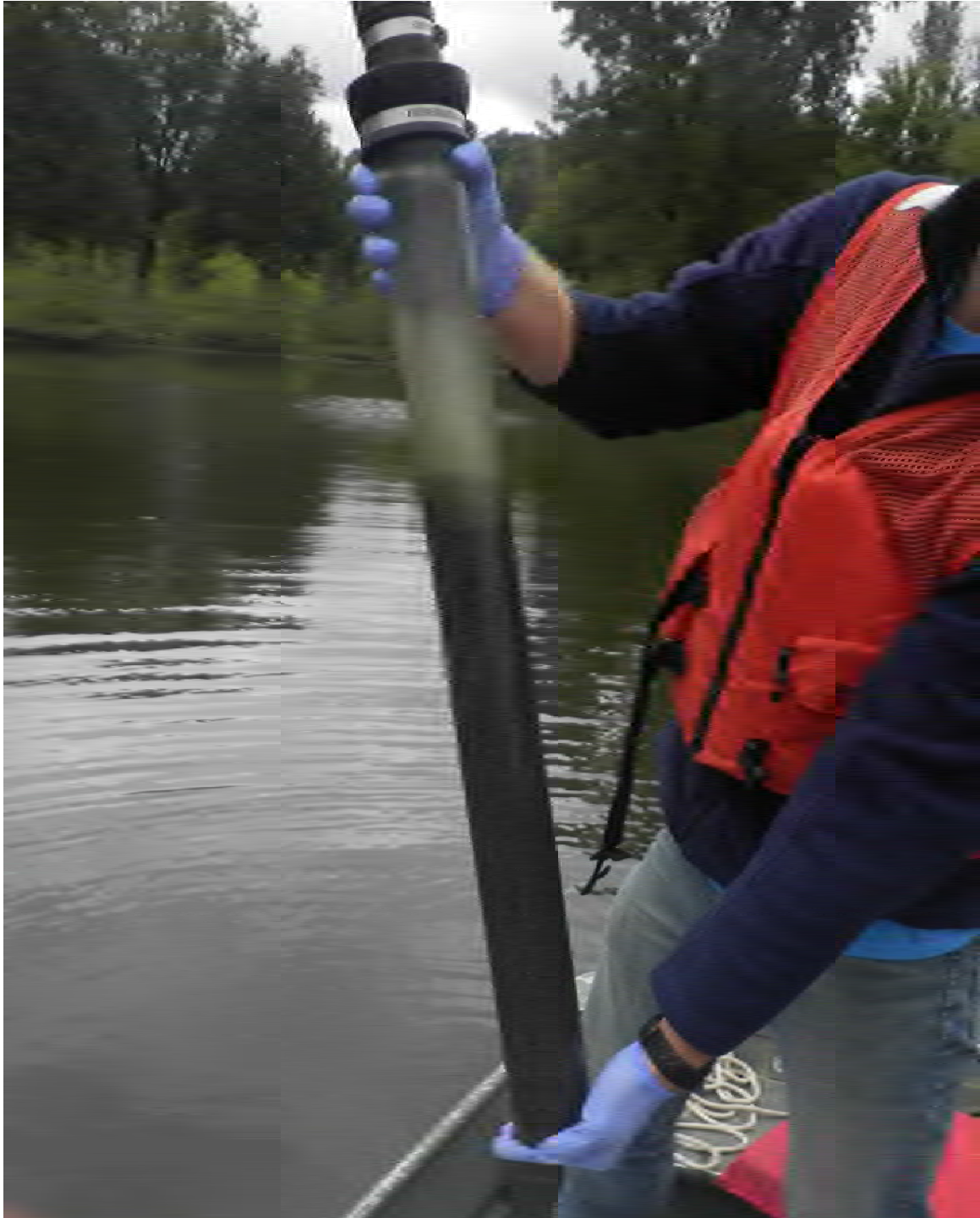
Photograph #2: Sediment core collected with push core sampling device.
