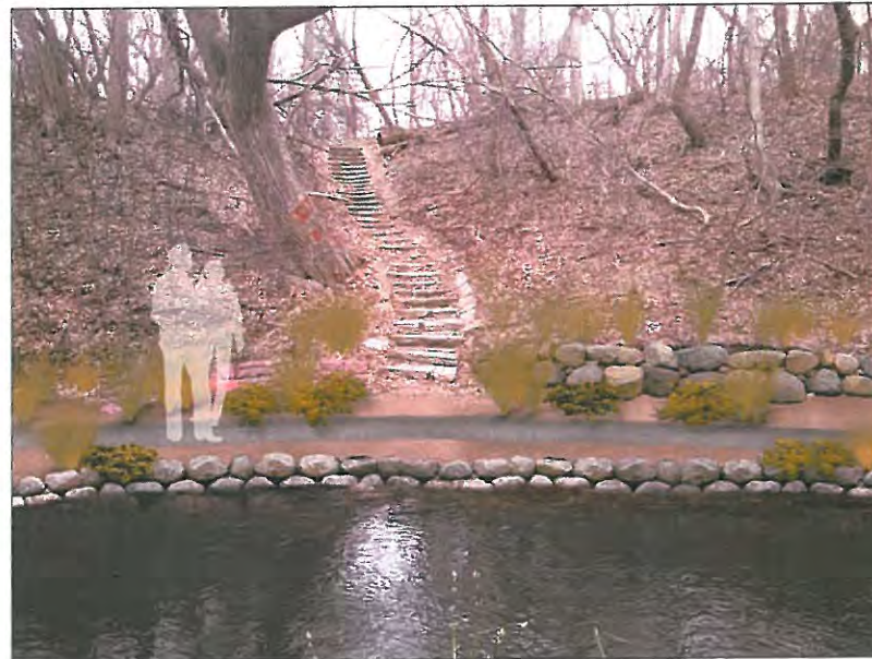
INSTALL BOULDER TOE STABILIZATION REPLACE RETAINING WALL AND REESTABLISH TRAIL
