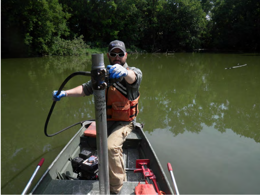
Photograph #1: Barr staff using vibra-core equipment to collect sediment core from Decola Pond B.
