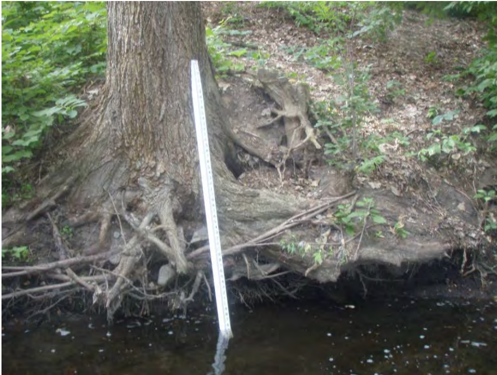
Photo 16. Site 10. Minor bank erosion with undercut trees.
