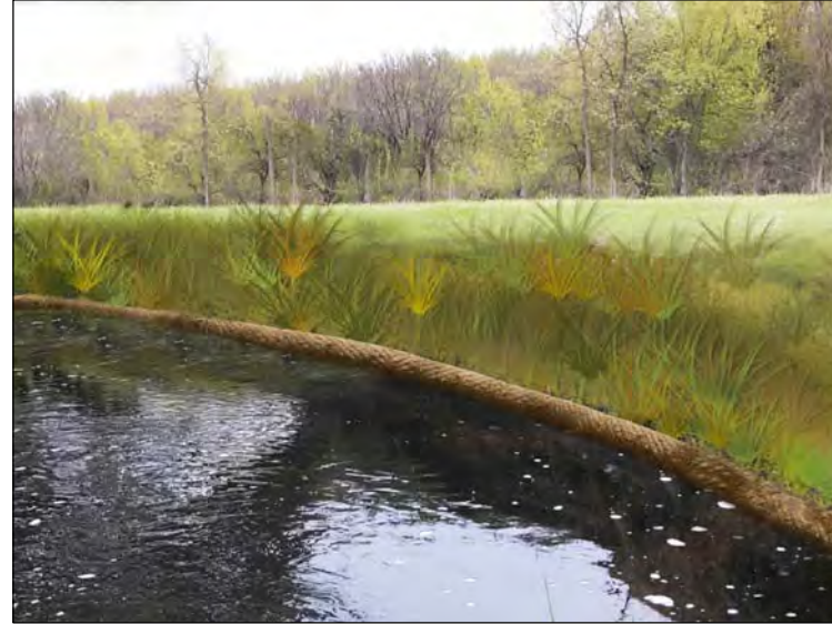
RESHAPE SLOPE AND INSTALL TREE REVETMENT
