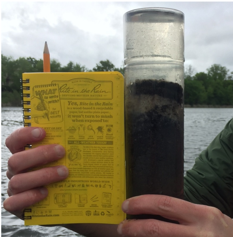
Figure 3 Photo of sediment core showing alum floc within the top layer
