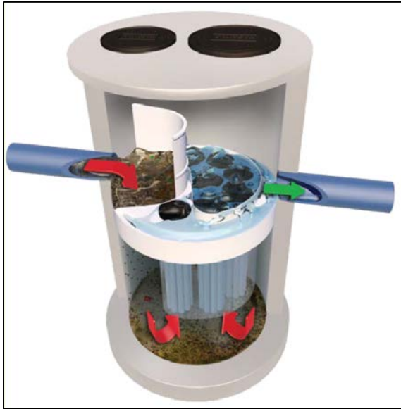
Figure 5: Contech Jellyfish Filter
