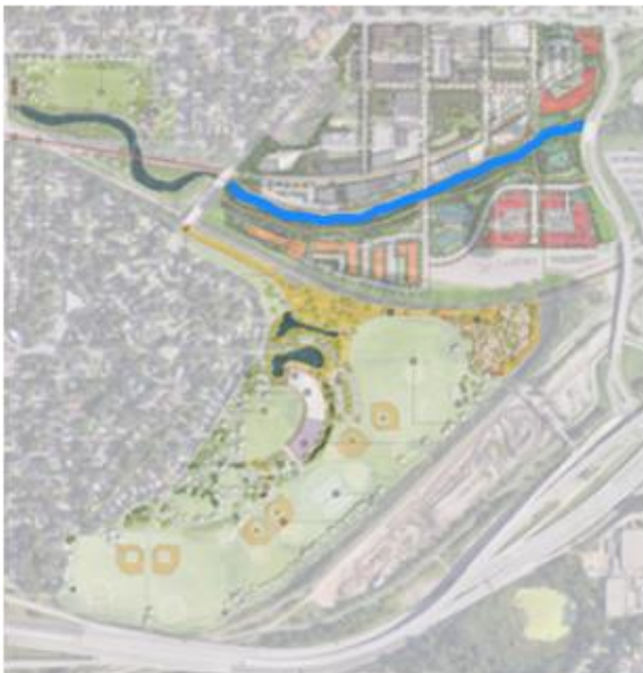
Proposed scenario under the 10-year storm event). Water would remain in low flow channel with trails accessible. No pooling within athletic fields.
