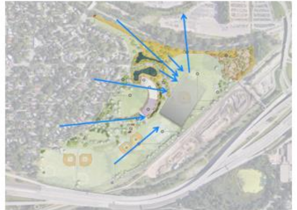
Proposed scenario under 100-year storm event. Rainfall directed to underground system, no impacts to athletic fields.
