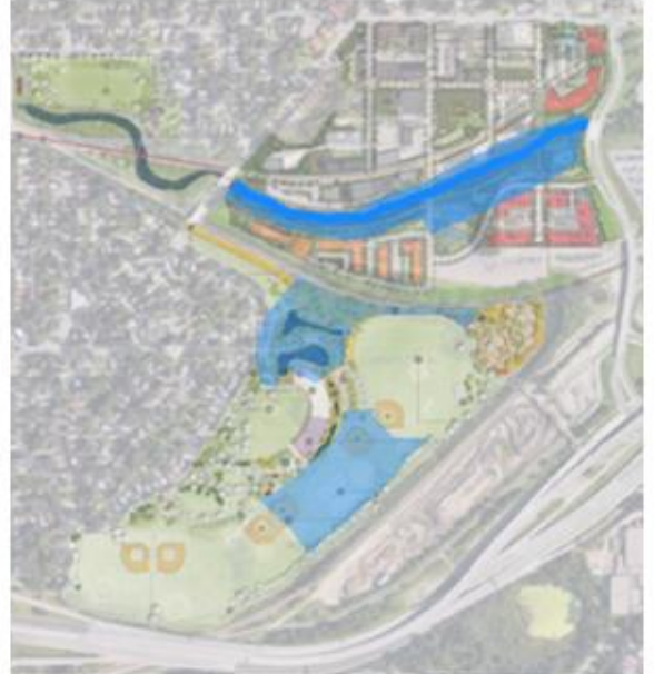
Proposed scenario under 100-year storm event. Flood would use entire channel, submerging trails and use surface storage in Bryn Mawr Meadows Park.
