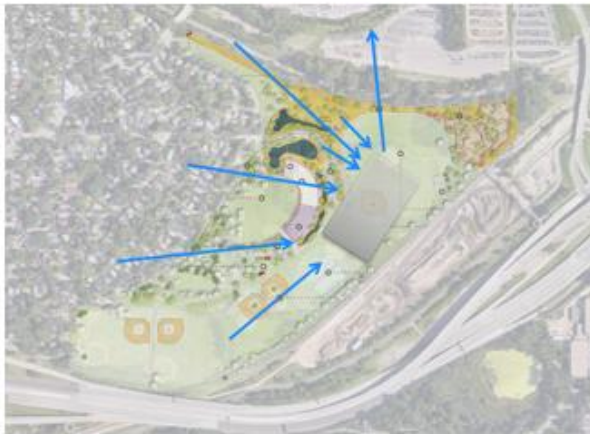
Proposed scenario under the 2-year storm event. Rainfall directed to underground system, no impacts to athletic fields.
