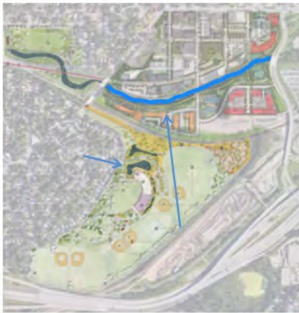
3. Proposed scenario under the 10-year storm event. Water would remain in low flow channel with trails accessible. No pooling within athletic fields.
