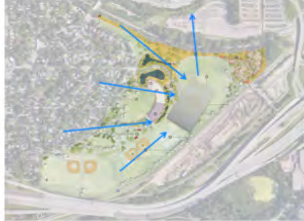
4. Proposed scenario under 100-year storm event. Rainfall directed to underground system, no impacts to athletic fields.
