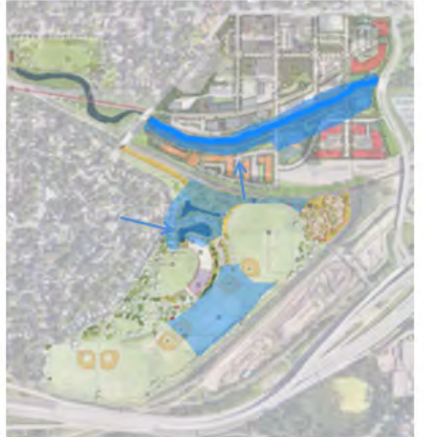
4. Proposed scenario under 100-year storm event. Flood would use entire channel, submerging trails and use surface storage in Bryn Mawr Meadows Park.
