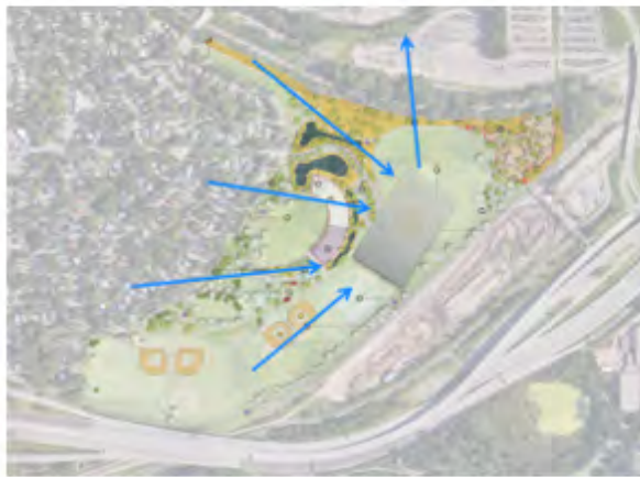
3. Proposed scenario under the 2-year storm event. Rainfall directed to underground system, no impacts to athletic fields.
