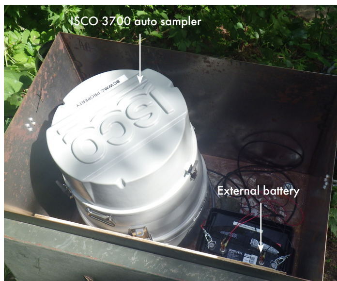
Figure 5: Automatic sampler and external battery
