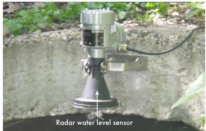
Figure 2: Radar water level sensor
