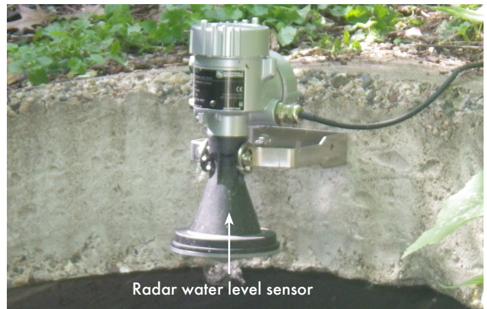
Figure 2: Radar water level sensor
