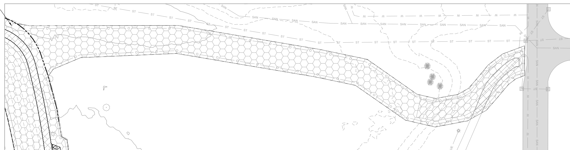
2 PLAN: ACCESS ROAD TEMPORARY WINTER EROSION CONTROL
