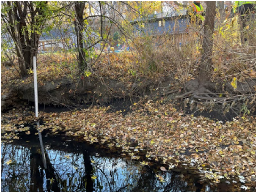
Photo 36: Site 3h. BEHI measurement at right bank of station 51+00 with undercut and deposition.
