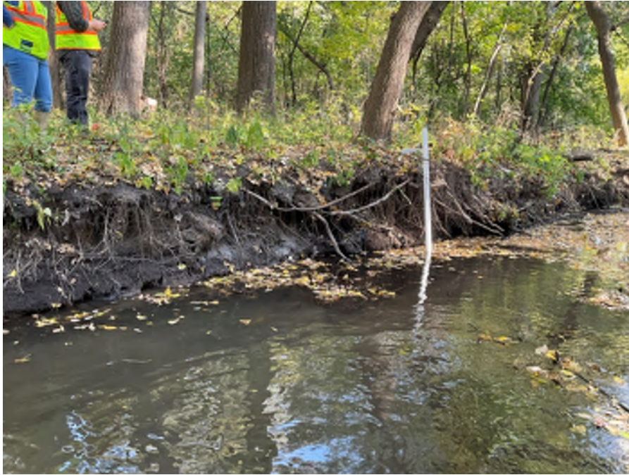
Photo 13: Site 2c. BEHI measurement and bare soil at the left bank of station 19+90 (facing downstream).
