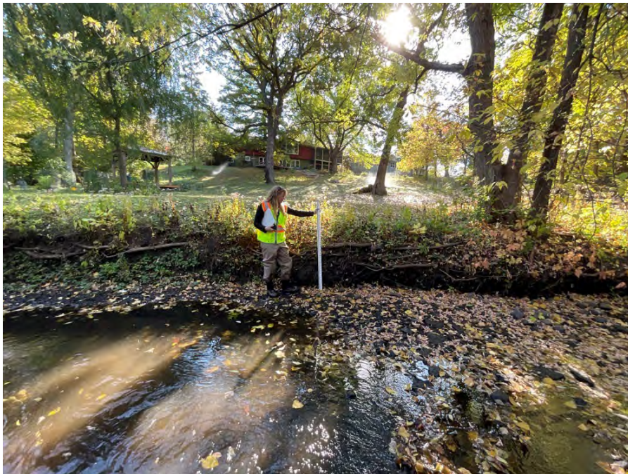
Photo 2: Site 1a. BEHI measurement at the right bank of station 1+60.
