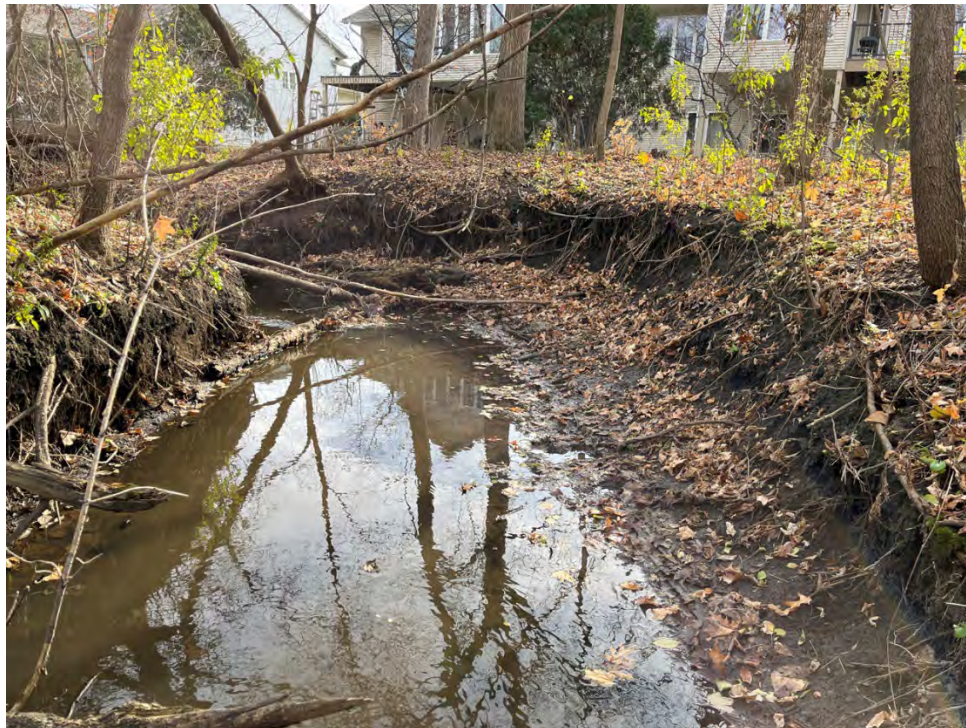
Photo 2: Site 1a. Looking downstream at station 2+75. The left bank is bare at a vertical angle, while the right bank is angled and has a soil material change at the bottom foot of the bank.
