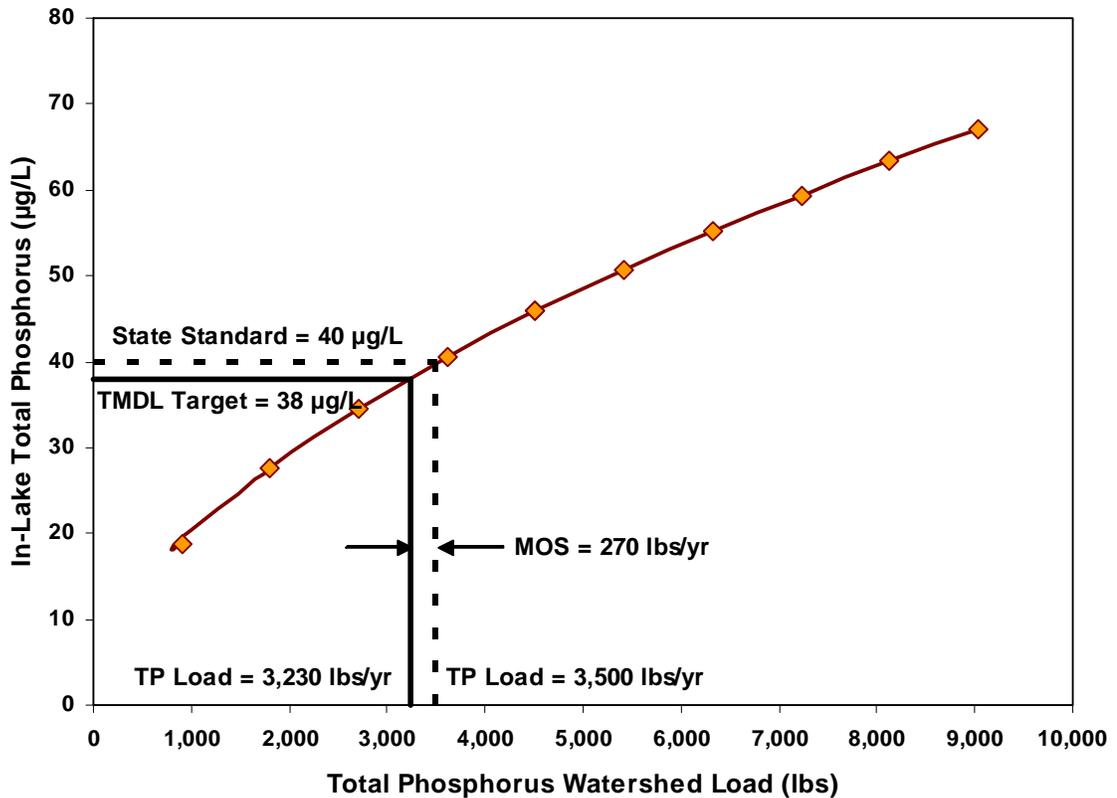
Figure 4-3. Determination of Explicit Margin of Safety.
