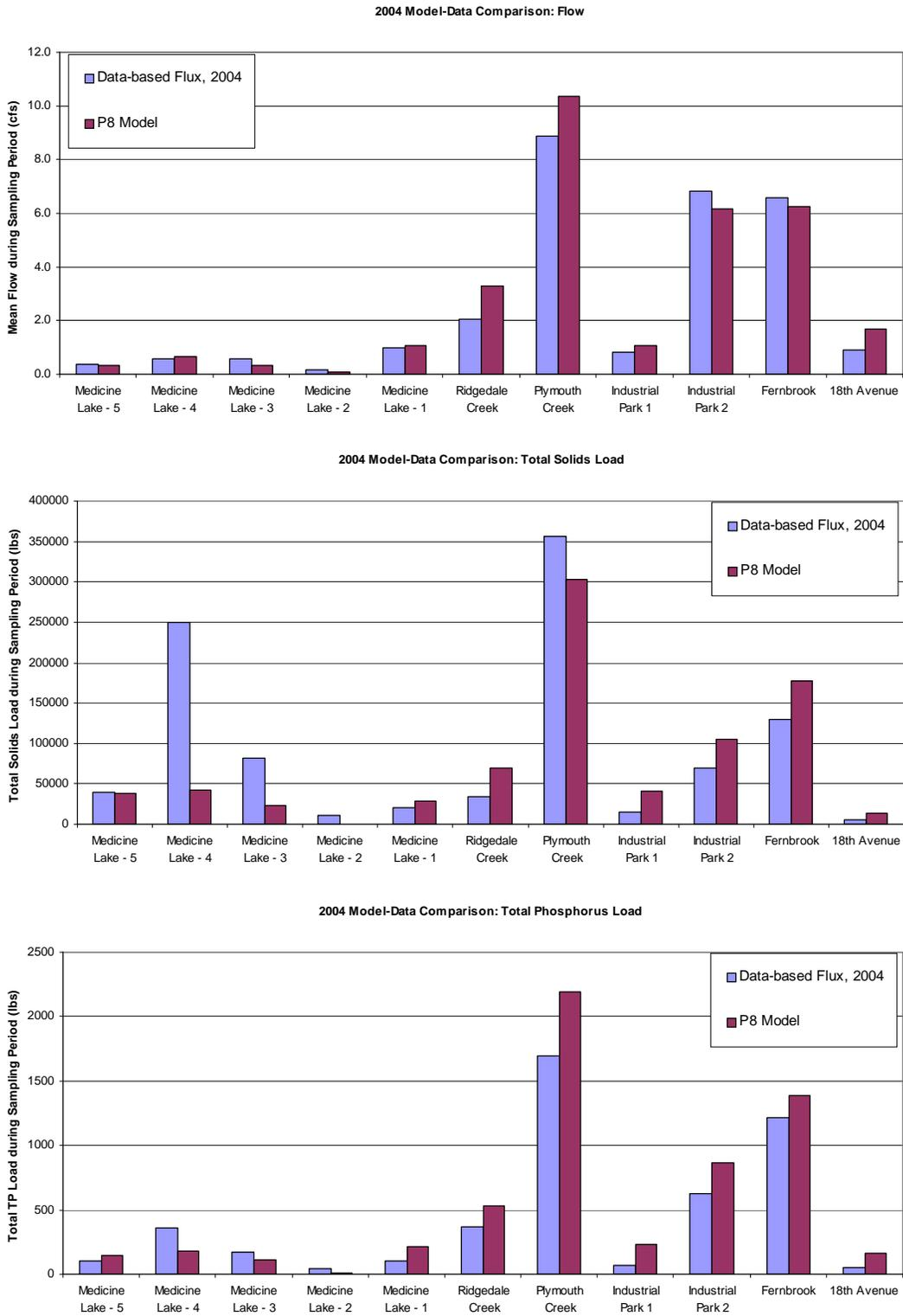
**Figure 8. Model-Data Comparison for 2004.**
