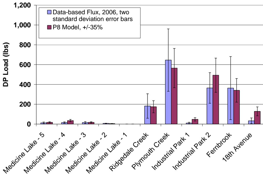
Figure 4. Model-Data Comparisons of DP for Calibration Year 2006.
