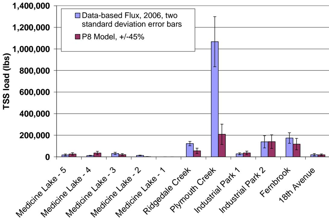
Figure 2. Model-Data Comparisons of TSS for Calibration Year 2006.
