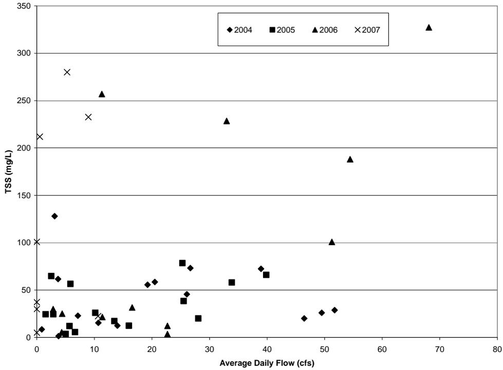
**Figure 5. TSS Versus Average Daily Flow Comparison for 2004-2007 Data at Plymouth Creek Site.**
