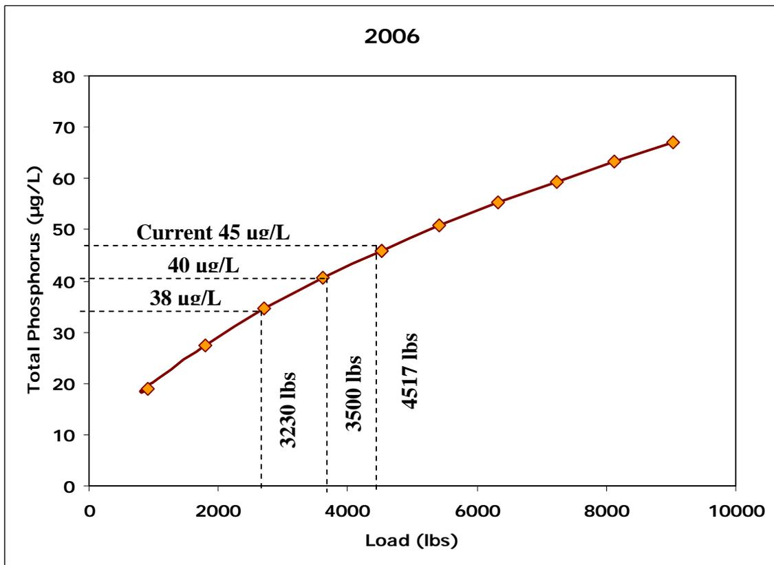
**Figure 12. BATHTUB watershed load response to in-lake TP concentration for 2006.**
